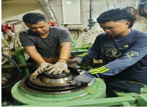
Gambar 3. Proses Membongkar *Purifier* Kapal MV.TANTO DAMAI
